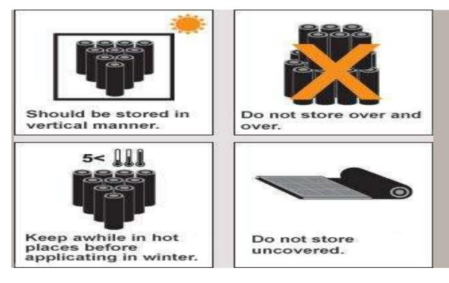
The rolls of bituminous membranes should be stored in vertical manner. Additionally during the transportation they should be placed vertically.
